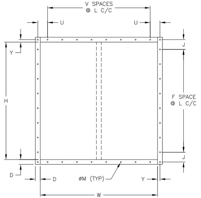
Standard Mounting Hole Pattern with Corner Holes
