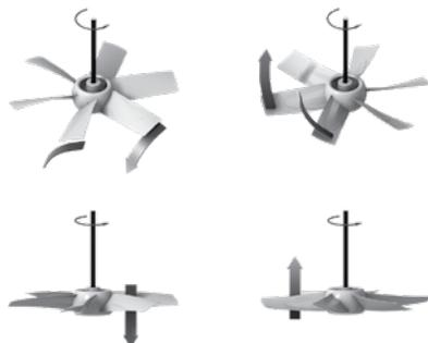
For 3-phase installations, fan rotation can be reversed by simply interchanging any two of the three electrical leads. For single-phase installations follow the wiring diagram located on the motor.
